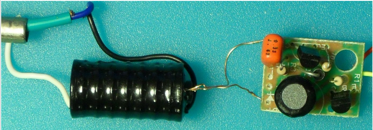
Fig.3 PCB and HV transformer
